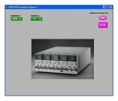
Step 2: If a device name appears on the Mainframe Info. it indicates the hardware is connected successfully.
